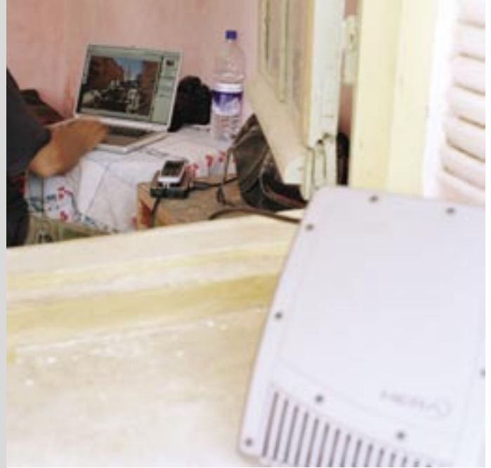
Working indoors in a safe and comfortable environment is made possible by connecting the separate interface unit and the antenna unit with a split cable.
